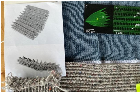
Knitting as a key technique to recreate sound-absorbing microstructures of moth wings Photo: Kateryna Basiuk
